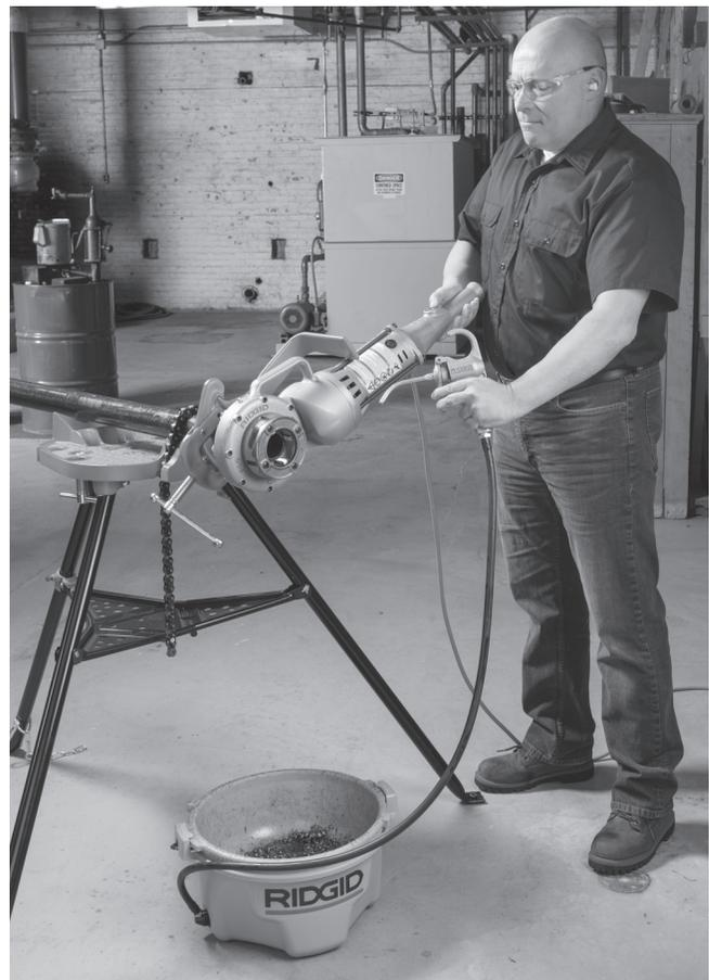
**Figure 9 – Threading Pipe**
