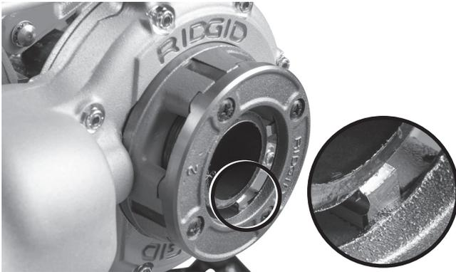
**Figure 10 – Pipe Even with Edge of Dies**
