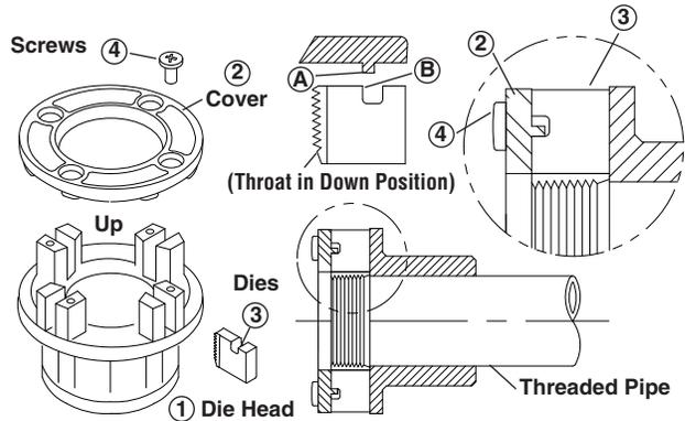
Figure 12 – Installing Dies in Die Head
