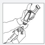
Remove the head by pulling the collar toward the base of the tool.
