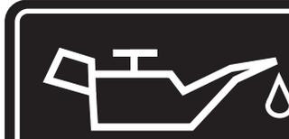
Add lubricant to full mark to start. Engine will not start or will shut off if lubricant is too low.
