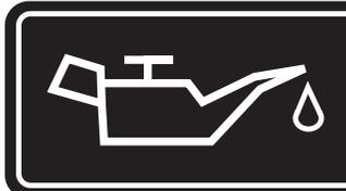
Add lubricant to full mark to start. Engine will not start or will shut off if lubricant is too low.
