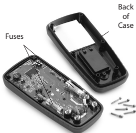
Figure 9 – Removing Back of Multimeter Case
