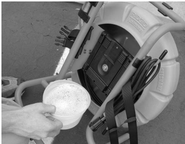
Figure 28 – Correct Cleaning Position
