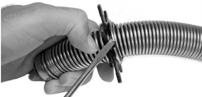
Figure 23 – Place flat tip of screwdriver between c-ring and base of spike and pry c-ring out of groove.
