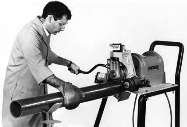
Figure 9 – Grooving Pipe While Exerting Light Hand Pressure Toward Operator
