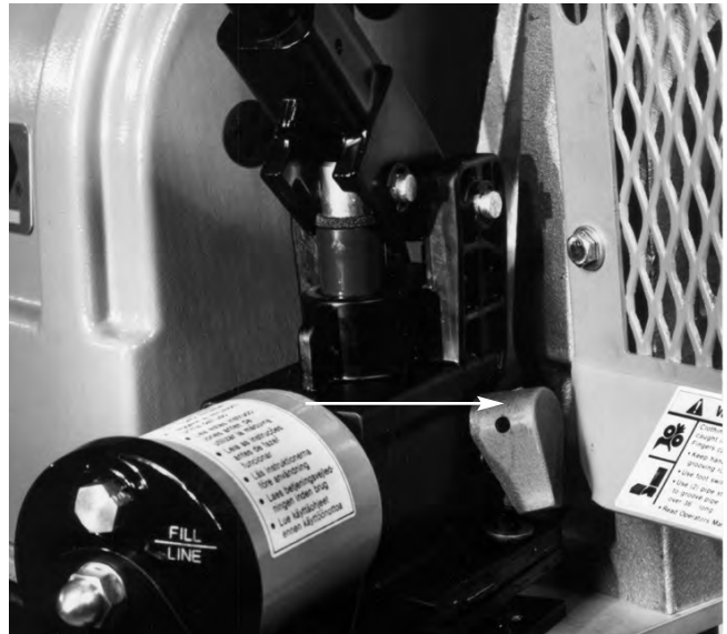
Figure 4 – Close-up of Release Lever on 918-I Pump
