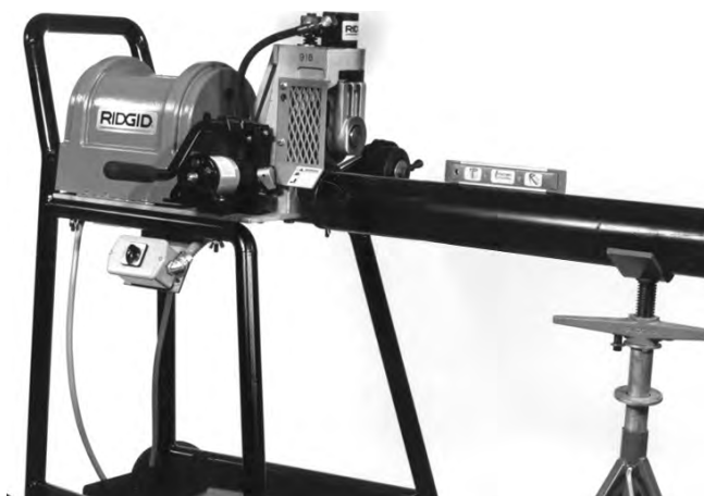
Figure 6 – Leveling Pipe on Pipe Support and 918-I Roll Groover
