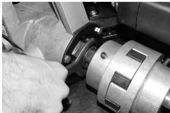
Figure 14 – Loosen and Remove Drive Shaft Retaining Nut
