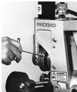
Figure 11 – Loosen Set Screw in Groove Roll
