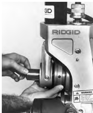
Figure 12 – Remove Groove Roll Shaft and Groove Roll
