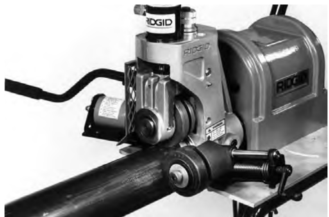
Figure 10 – Adjusting Pipe Stabilizer
