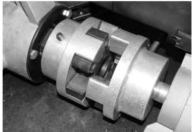
Figure 16 – Removing Bearing, Retaining Nut and Front Half of Coupling
