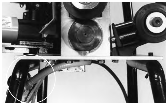
Figure 20 – Removing Base Assembly From Stand
