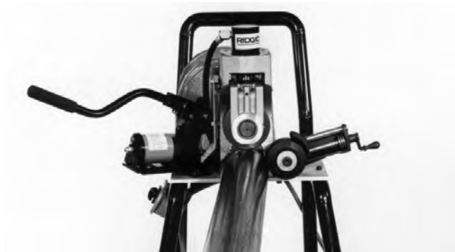
Figure 7 – Offset Pipe on 918-I (exaggerated for clarity)
