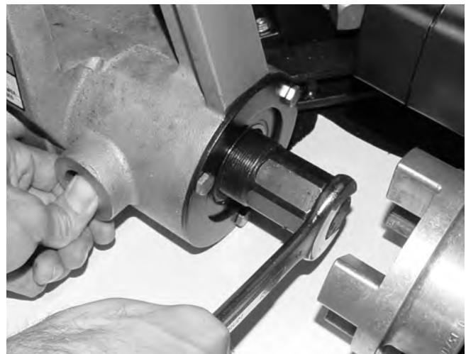
Figure 17 – Engaging Spindle Lock and Loosen Draw Bolt
