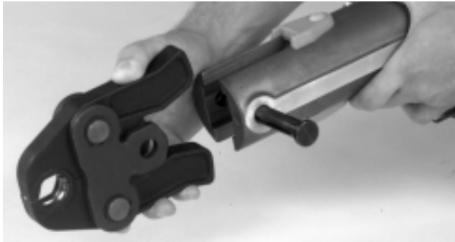
Figure 3 – Sliding Jaw Set Into CT400
