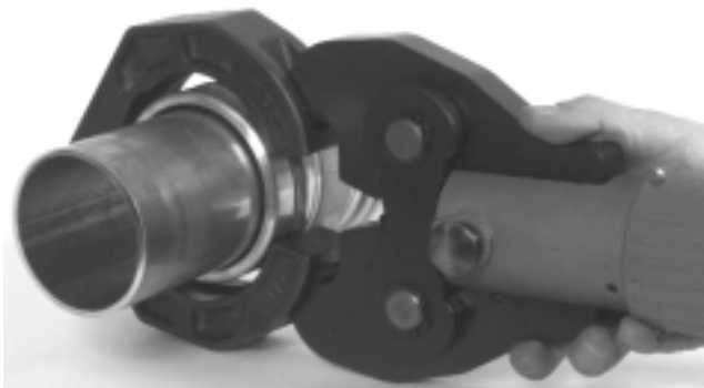
Figure 9 – Attaching Ring Actuator To Press Ring
