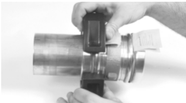
Figure 8 – Installing Press Ring Onto Fitting
