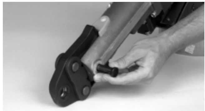
Figure 2 – Pulling The Jaw Set Mounting Pin Out
