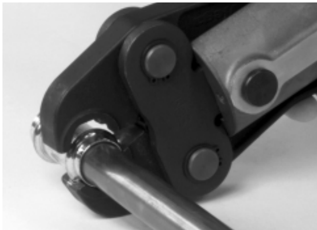
Figure 5 – Placing Scissor-Style Jaw Set Around Fitting
