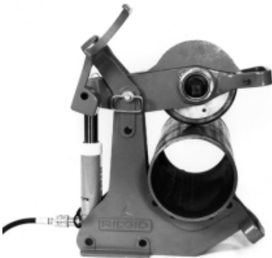
Figure 8 – Positioning Pipe in Cutter
