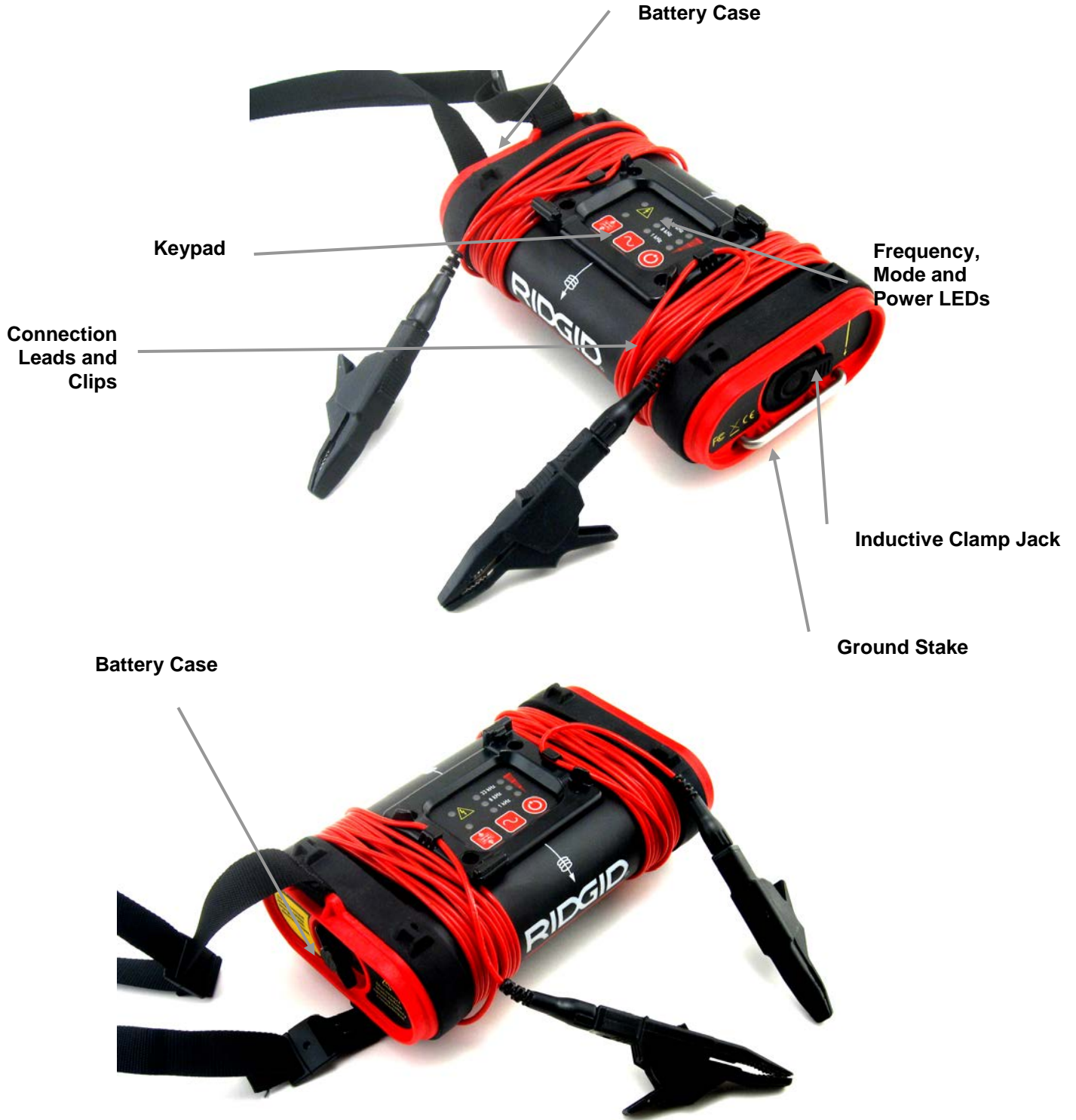
Figure 1: Components of the NaviTrack Brick
