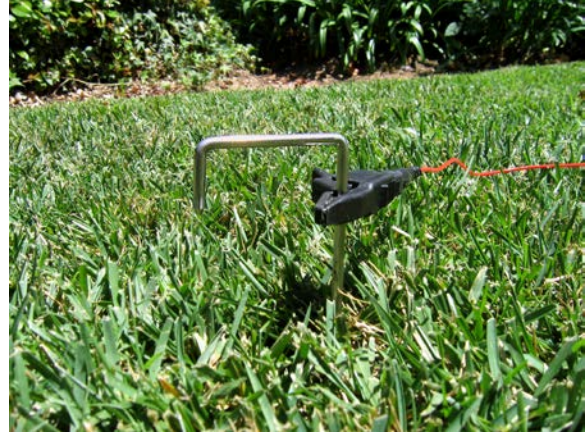
Figure 4: Connecting the Ground Stake
