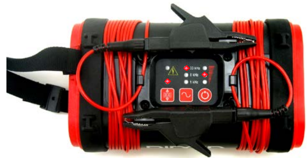
Figure 11: NaviTrack Brick in Inductive Mode at 33 kHz
