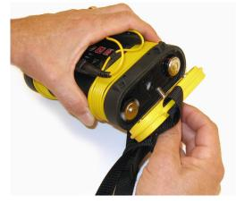
Figure 4 – Removing the Battery Cover
