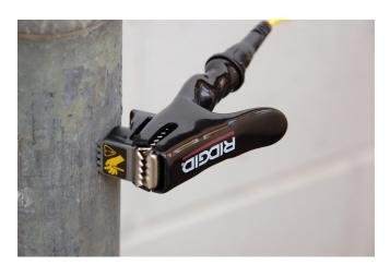
Figure 7 – Connecting the ST-305 using the magnet
