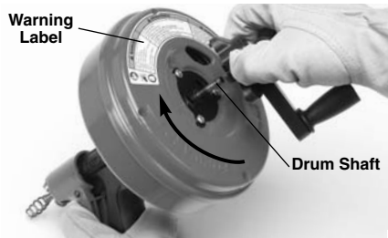
Figure 2 – Removing Crank Handle From Power-Spin
