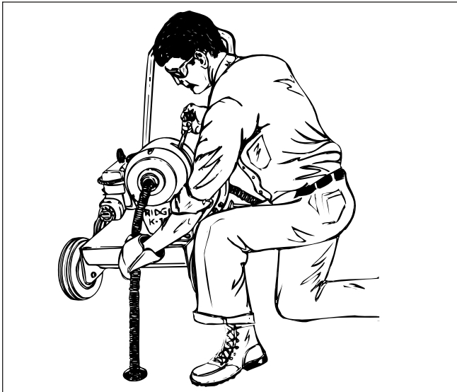
Figure 5 – Operating Drain Cleaning Machine
