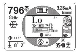
If more than one Bluetooth enabled SeekTech transmitter is present, press the Left Arrow key • to cycle through available transmitters. Press the serial number listed below the transmitter icon to identify the specific transmitter you want to control.
