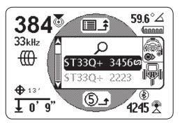
Once a connection is made, the transmitter automatically powers on. When connected, the Bluetooth icon  $\[mathbb{B}\]$  is visible on both the transmitter's and the receiver's screens. On the transmitter, a chain link image confirms that the two units are connected.
