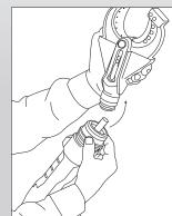
Remove the head by pulling the movable collar toward the base of the tool.
