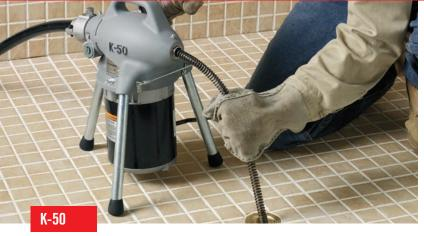
The Professional's choice since 1957 because of its power and versatility. Use  $\frac{1}{8}$ " cables for  $\frac{1}{4}$ " to  $\frac{1}{4}$ " lines. Add the A-17 adapter for  $\frac{3}{4}$ " to  $\frac{2}{4}$ " sink lines.
