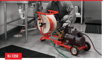
1350 PSI and a two-sided pulse action makes for fast effective cleaning of lines.
