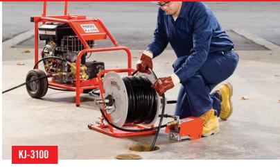
The 16 HP gas engine provides up to 3000 PSI to easily clear main lines from 2" to 10".
