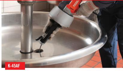
The K-45 family of drain guns are the professionals' choice for cleaning small secondary drain lines from ¾" to 2½".
