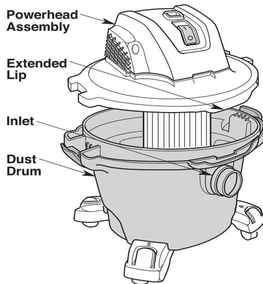
2. Press in on the two Latches located on either side of the Dust Drum until they snap into place, securing the Powerhead Assembly to the Dust Drum.
