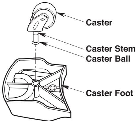
4. Place Caster Foot w/Caster over post on bottom of Dust Drum and press firmly in place, as shown.
