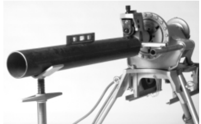
Figure 5 – Leveling Pipe On Pipe Support and 960
