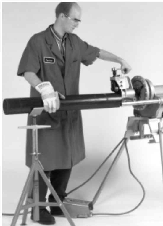
Figure 9 – Applying Pressure On Pipe with Power Drive In REVERSE Mode
