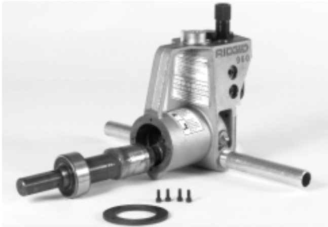
Figure 11 – Removing Drive Shaft From 960
