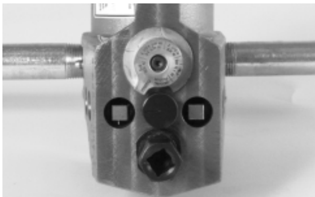
Figure 8 – Close-Up Of Integral Index Depth Gauge In Grooving Position
