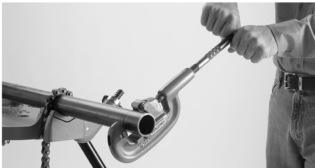
Figure 1 – Cutting End of Pipe
